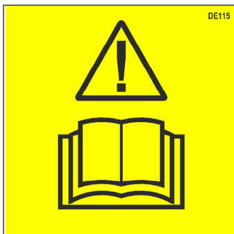
Figure 3: Read Owner's Manual Warning (DE115) • Located at components that require operator adjustment. • See Owner's Manual for information on components requiring operator adjustment.
