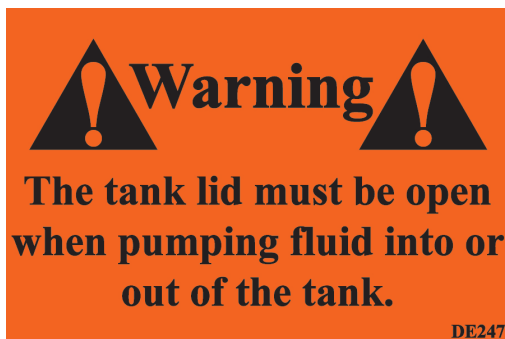
Figure 5: Open Tank Lid when Pumping Fluid into or out of Tank • Located at tank lid and pump.
